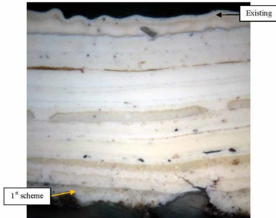
Photomicrograph of BIC/13 (x 200 digitally reduced) Building 89: South front. R/H lower window cill
